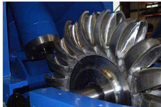
This Canyon Hydro Pelton-type turbine runner is similar to the design for the Boulder Canyon Hydroelectric Project.
